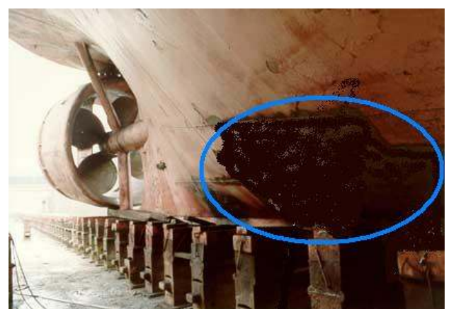
Figure 2: Ship hull with degradation area.
